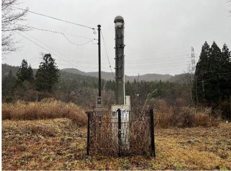
A photograph of a crustal movement measurement device. It consists of a tall, cylindrical metal structure mounted on a concrete base, enclosed within a black metal fence. The device is located in an open field with some dry grass and trees in the background. |
